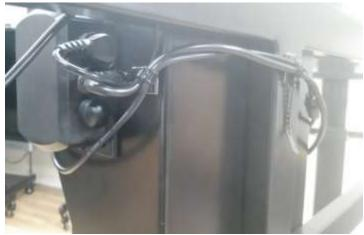
• Install the Din4 Extension Cable into the 4 pin connector on the Controller. Route the Din4 Extension Cable around the front of the Screen Mounting Frame (3) and connect to the Din4 Cable from the Extrusion (2). Secure the cable using the Cable Clip on the front of the Screen Mounting Frame (3)
